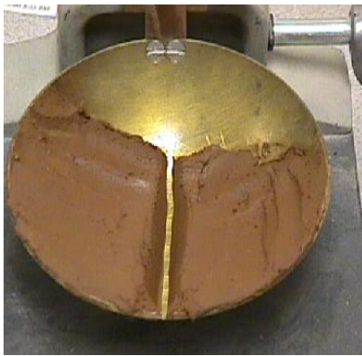
Fig 3.1 Groove in the soil sample using grooving tool for moisture content at Cecos lab
