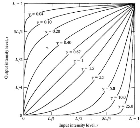
Fig. 7. Plots of eq. 1 for  $c=1$  and varying  $\gamma$  [5]
