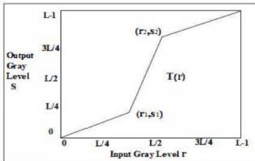
Fig. 10. Plot for Contrast Stretching [12]
