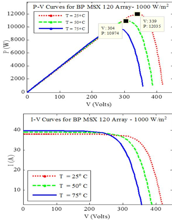
**Fig. 6:** BP MSX 120 Array Characteristic Curves as a Function of Solar Irradiance (G)
