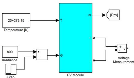
Fig. 3: Block Diagram of PV Module
