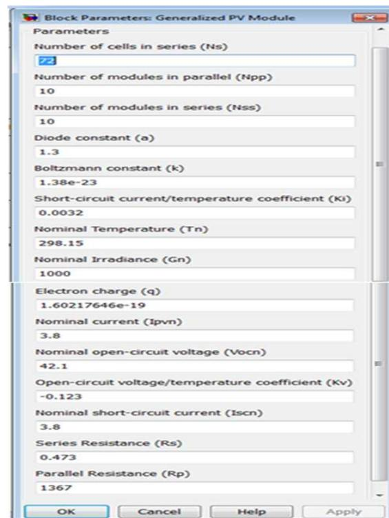
Fig. 4: Mask for Generalize PV Module
