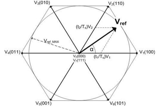
Fig. 5: Space Vector Corresponding to Each Switching States [16]
