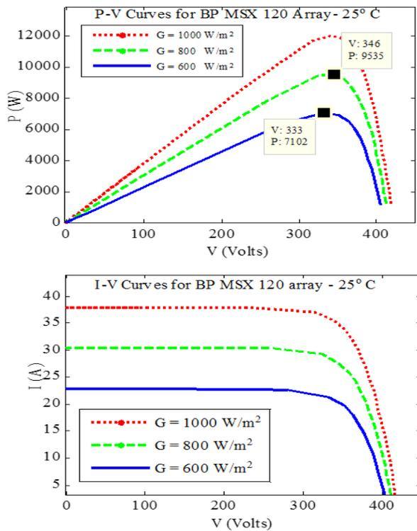
**Fig. 7:** BP MSX 120 Array Characteristic Curves as a Function of Temperature (T)
