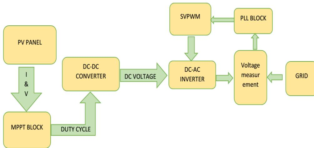
Fig. 1: Block Diagram of Solar PV System
