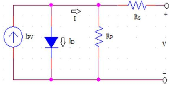
Fig. 2: Single Diode Model of a PV Device
