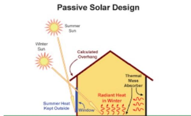
Figure 1: Passive Solar Technique
