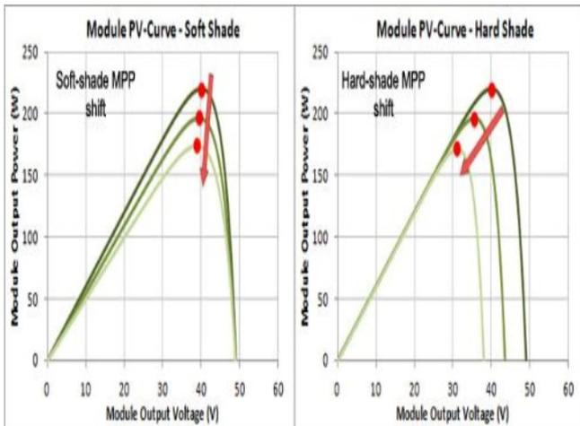
Due to disturbance in power generation, there is a need of Bypass circuits which can improve the efficiency of solar system. Effect of soft shade observed practically is shown in table 6.
