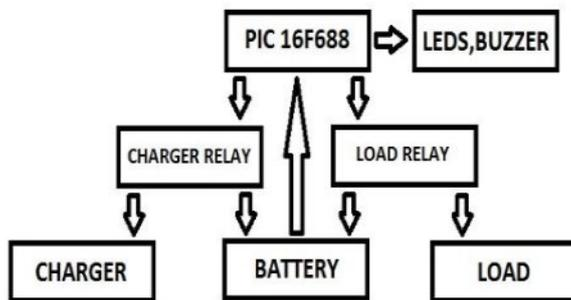
Figure 5 charging and discharging control
