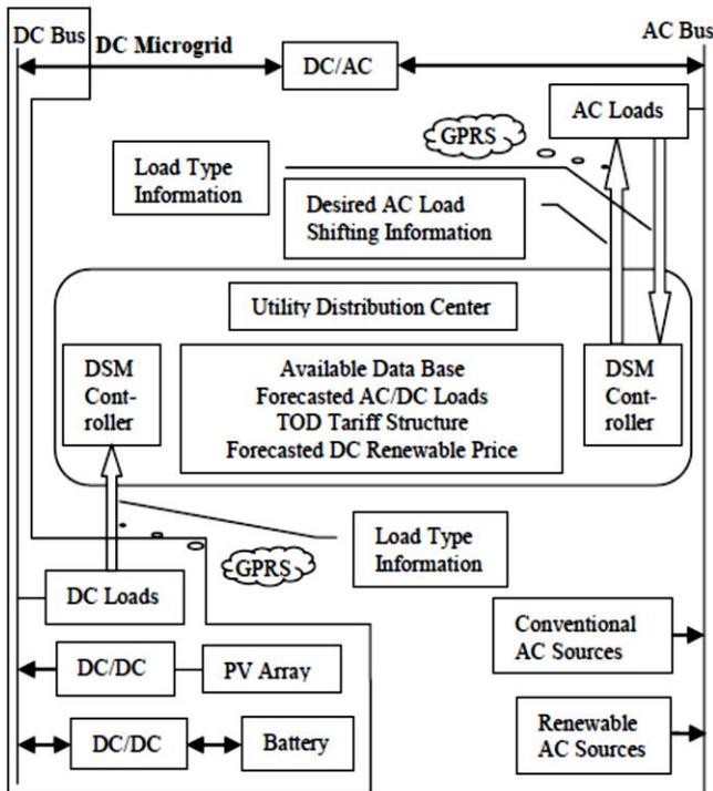
Figure 2. Architecture of proposed DSM [7]
