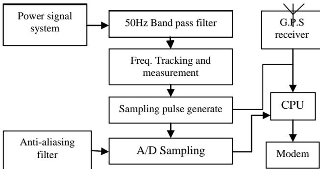
Figure 2: Typical Structure of Phasor measurement unit (P.M.U)
